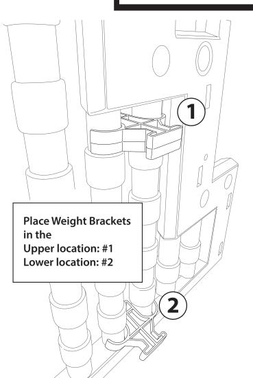
Attach the weight brackets to each side of your pool step.
