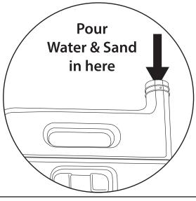
Fill each of the 2 side weights with sand. This is what gives the weight system it's weight. First pour approximately 10 ounces of water into the step. Then pour filter sand into the spout until it is full.
