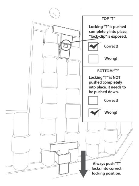
To lock the weigh brackets in place you must use the locking T's. Simply slide the locking T through the square hole in the bracket that is protruding through the step side inside the step. Push the "T" all the way down until it locks in place.
