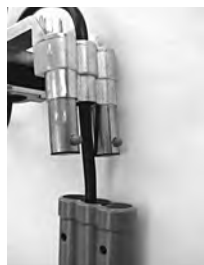
Detaching housing from bracket
